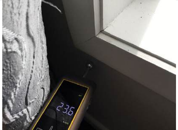
14. Typical low moisture reading below windows
