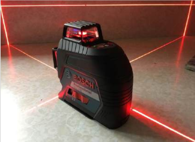
13. Floor levels checked with laser level
